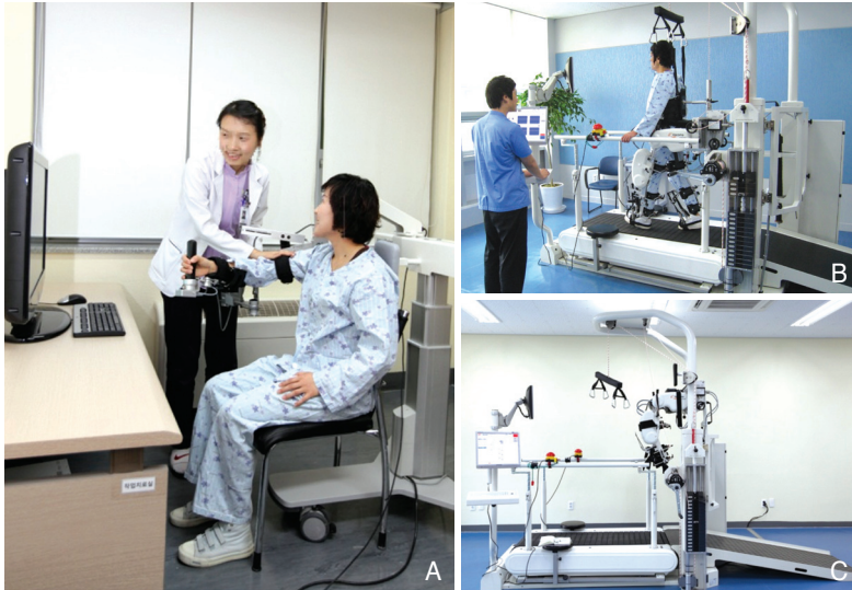
Figure 1. (A) Person with stroke engaged in robotic therapy using Armeo (B) Person with stroke engaged in robotic therapy using Lokomat (C) Lokomat (Hokoma AG, Zurich, Switzerland)
