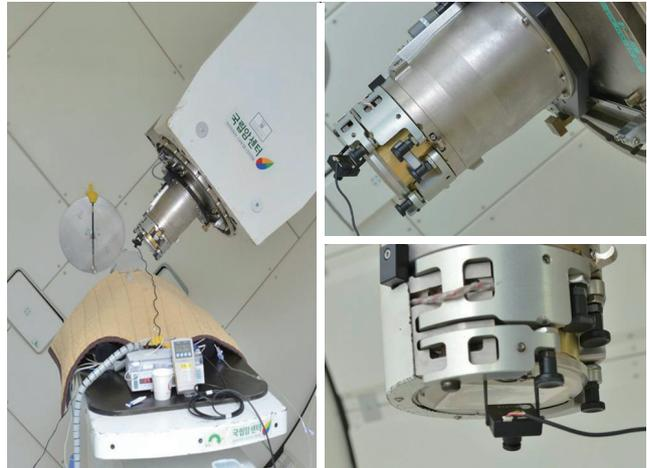
**Fig. 4.** Treatment monitoring system used at National Cancer Center, Korea. The position of the eye is monitored in the control room through a CC camera attached to the aperture during treatment. CC, closed-circuit.
