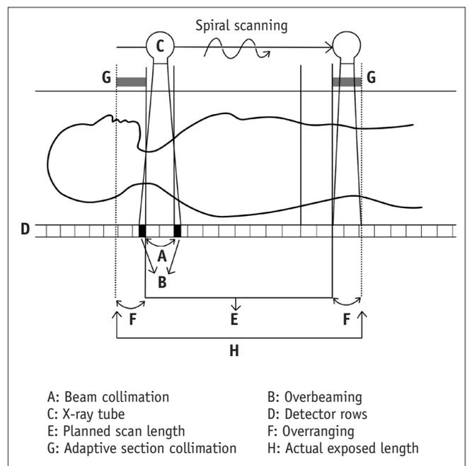
**Fig. 2.** Diagram illustrating overbeaming, overranging, and adaptive section collimation technology during spiral scanning.
